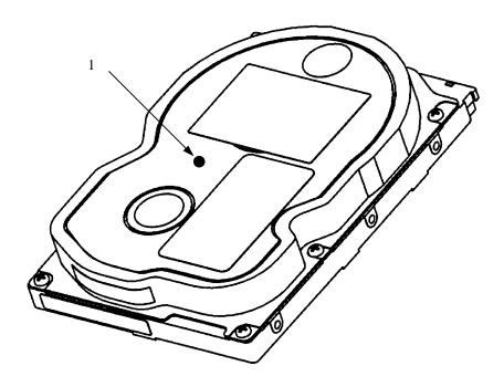
Figure 3.6 Surface temperature measurement points
